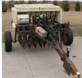
Width 72" Disc Diameter 18" Disc quantity 20 Disc spacing 7 - 1/2" Approximate weight 818 lbs. Tractor hitch Cat. 1 Tractor engine hp 32 - 70 hp
